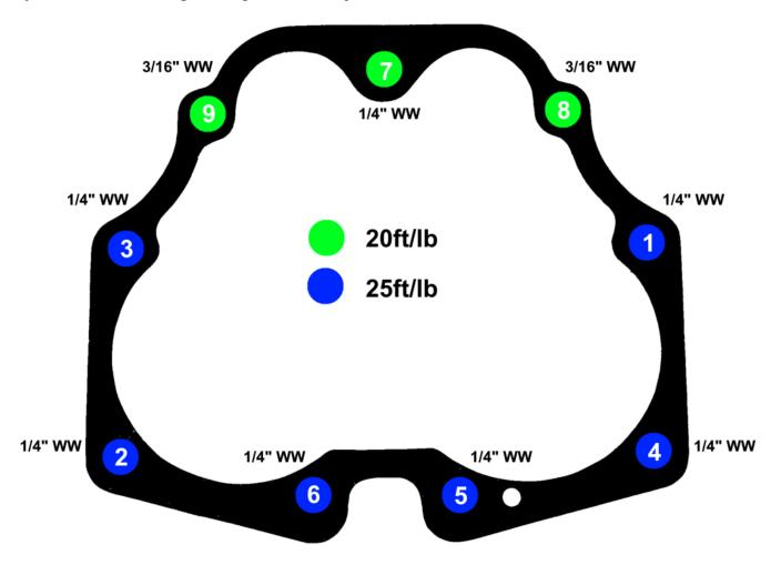
Cylinder Base 750 Tightening Order, Torque, and Wrench Size 1972/3:
